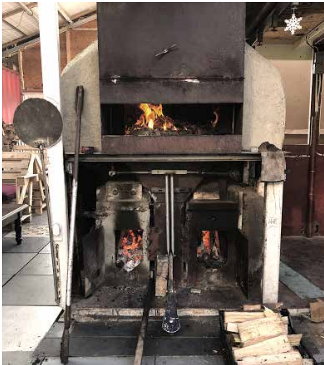
Fig 3.43, Front view of the Pizza oven with a system of two batch-burners below, Fig 3.44, Pizza oven in action Photos by KasKantine
